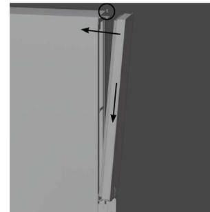
7. Now turn the door 180° and reinsert it into the hinge at the bottom and fasten the screw on the upper hinge.
