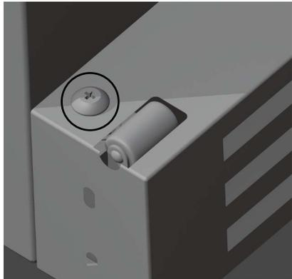
3. Now adjust the guide roller so that the door does not stop when closing, but runs slightly onto it.
