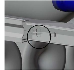
2. Press the plastic tab on the left upwards and on the right downwards and pull out the shelf at the same time.
