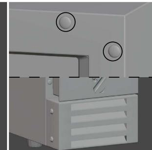
8. Reinstall the rubber covers and the front ventilation grille.
