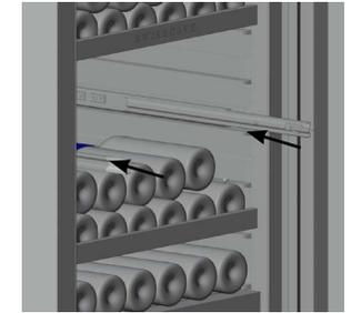
3. To reinsert, push back the pull-out rails, slide the shelf into the rails on both sides and push it in as far as it will go.
