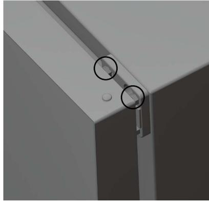
2. Then slightly loosen the hinges using a size 8 open-end wrench, align the door properly and retighten the screws.
