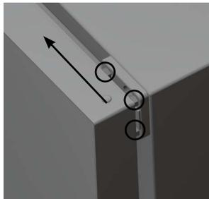
3. The hinges can now be released using a size 8 open-end wrench and then extended to the left together with the door and unhinged.
