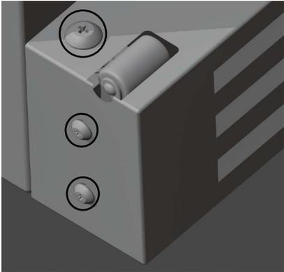
1. First remove the plinth grille. To do this, loosen the screw on the guide roller and the 2 Phillips screws on both sides of the base grille.
