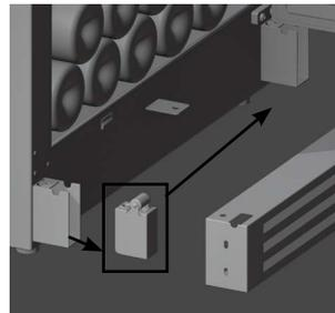
5. Now transfer the guide roller insert to the other side (must be opposite the hinge side at the end) and fit the plinth grille.
