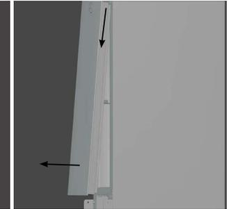
3. Carefully pull the glass door out of the hinge at the bottom and now drive the glass door down out of the upper guide.
